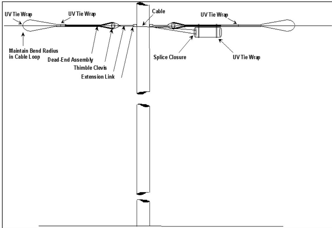
**Figure 14** – Cable storage loop using tie-wraps. This storage method is generally used for distribution applications or for transmission line applications where e-field space potentials are < 12 kv and where tracking resistant sheath materials are not required.
