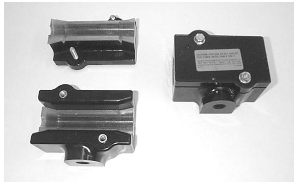
**Figure 3 - Intermediate Suspension Attachments – used between dead ends for span lengths up to 600 feet and for line angles up to 20° due to changes in elevation or direction.**
