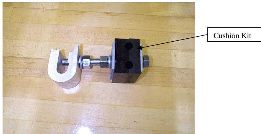
Figure 6 – Download Cushion Kits for use on either wood pole, concrete, or steel structures. The figure below is the set up for steel lattice towers. For wood poles applications, the cushion kit, washer, and a lag screw are used.
