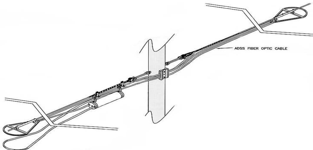
**Figure 15** – Cable storage using “snow-shoes”. This storage method is generally used for distribution applications or for transmission line applications where e-field space potentials are < 12 kv and where tracking resistant sheath materials are not required.
