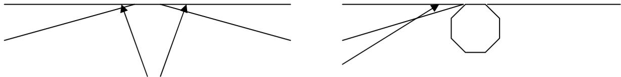
**Figure 8 – The arrows indicate a 10° maximum line angle change on either side of intermediate attachment hardware (total line angle change up to 20°) or 15° maximum line angle change on either side of heliformed suspension hardware (total line angle change up to 30°).**
